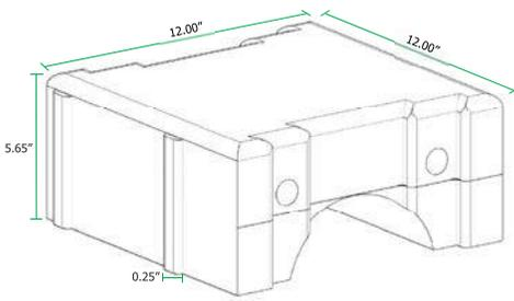
The PavDrain block is 12" x 12" but also has two 0.25" Spacer Tabs on each side of the block. Please consider these when measuring.
